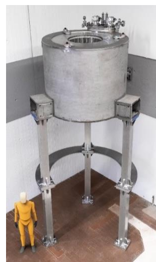
Fig. 1: The TUHH vertical MRI magnet.
